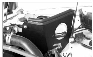
11. Using the provided hardware, secure the heat shield to the original air cleaner mounting holes
