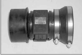
15. Install the filter adapter onto the mass air sensor as shown
