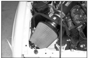
23. Install the K&N $^{\circ}$  air filter onto the filter adapter and slide the vent hose through the hole in the heat shield.
