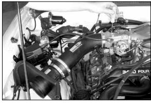
17. Slide the K&N<sup>®</sup> intake tube into the mass air adapter, then secure the other end onto the throttle body as shown.
