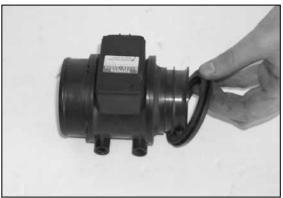
2. Disconnect the mass air sensor electrical connection.
