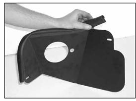
8. Apply the trim seal to the heat shield as shown. NOTE: Some trimming of the edge may be necessary
