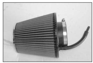
22. Install the vent hose with hose menders from step #19 into the K&N<sup>®</sup> air filter as shown. NOTE: On vehicles NOT equipped with an EVAP line attached to the airbox, install the hose mender with vent cap into the filter; the vacuum line will not be used.
