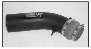
13. Install the 1/4" npt fitting onto the K&N $^{\circ}$  intake tube as shown.
