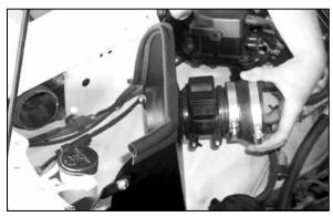
16. Install the mass air sensor assembly into the hole on the heat shield as shown.
